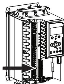
Push the card carefully into the expansion slot, then press firmly into the internal connector.
