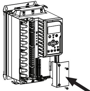
Replace the cover and screw firmly in place.
