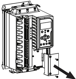
Remove the two screws holding the expansion card cover in place, then remove the cover.
