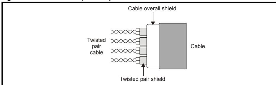
Using this type of cable allows for the connection of the outer shield to ground and the inner shields to 0V at both the drive and encoder.
