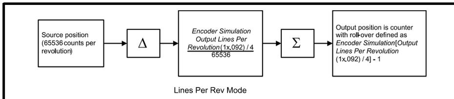
If *P1 Position (1x.029)* is selected as the source and *Encoder Simulation Incremental Mode Select (1x.091) = 0* then the input and output counters are synchronised at power-up and when the P1 position feedback interface becomes initialized, so that the output marker is synchronised with zero position for the P1 position feedback interface. For devices that support a marker, the effect of the marker on the position can be selected using *P1 Marker Mode (1x.031)*.
