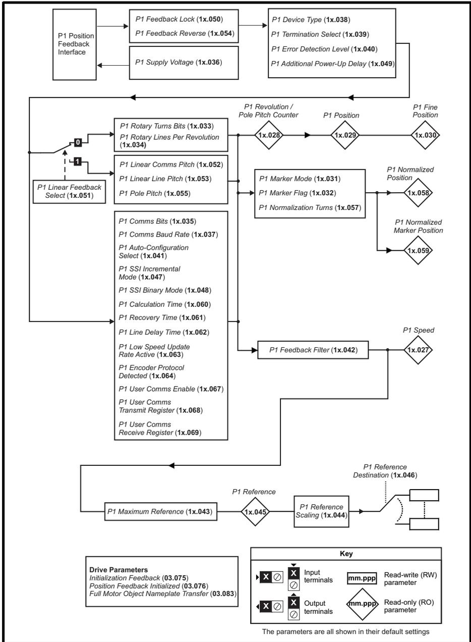
**Figure 7-2 P1 Encoder Simulation Output**
