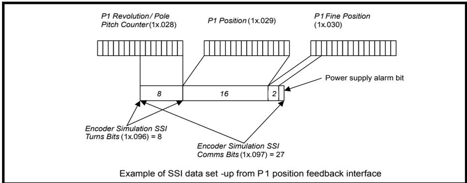
The SSI output is then clocked out from the register as shown in Figure 7-7.
