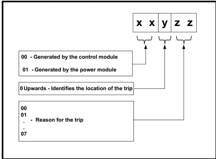
For example, if the drive has tripped and the lower line of the display shows 'OHT Control.2', with the help of Table 13-3 below the trip can be interpreted as; an over temperature has been detected; the trip was generated by fault in the control module, the control board thermistor 2 over temperature. For further information on individual sub-trips, refer to the diagnosis column in Table 13-4.
