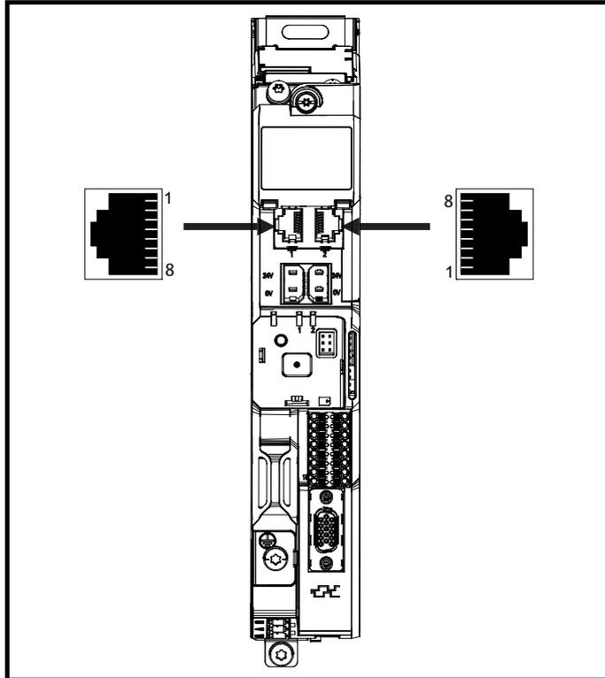
The M750 provides two RJ45 connections with an Ethernet switch for easy network creation.
