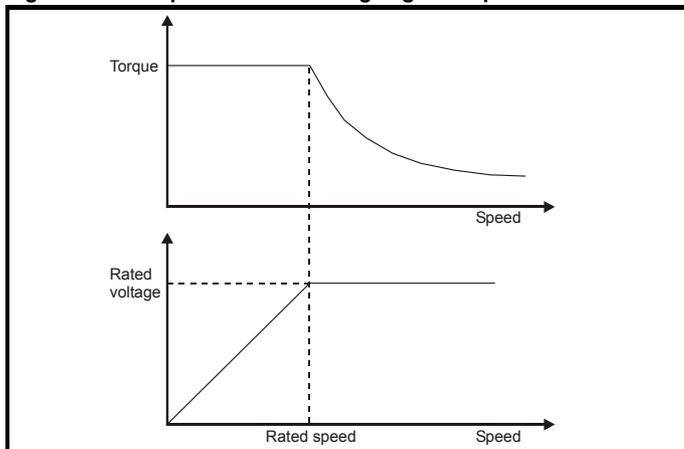
Care must be taken to ensure the torque available above base speed is sufficient for the application to run satisfactorily. The saturation breakpoint parameters (Pr **05.029**, Pr **05.030**, Pr **05.062** and Pr **05.063**) found during the autotune in RFC-A mode ensure the magnetizing current is reduced in the correct proportion for the specific motor. (In open loop mode the magnetizing current is not actively controlled).
