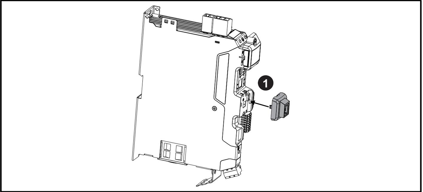
1. Align the KI-Remote Keypad Adaptor to the display housing and push on until it clicks into place.
