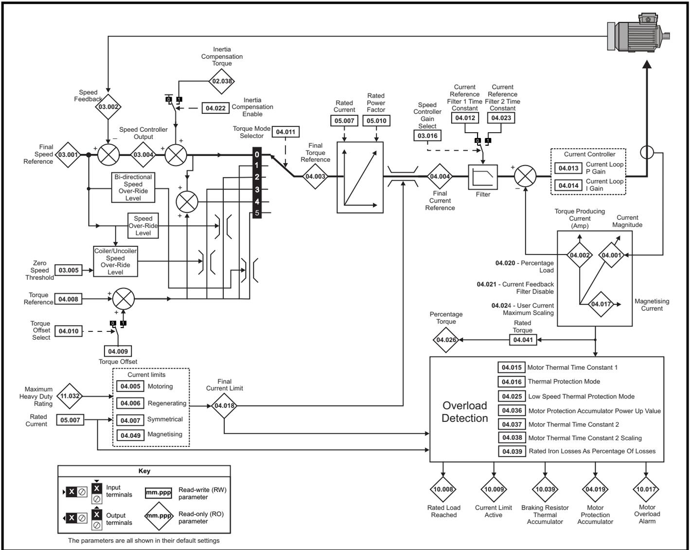
Figure 12-12 Menu 4 RFC-S logic diagram
