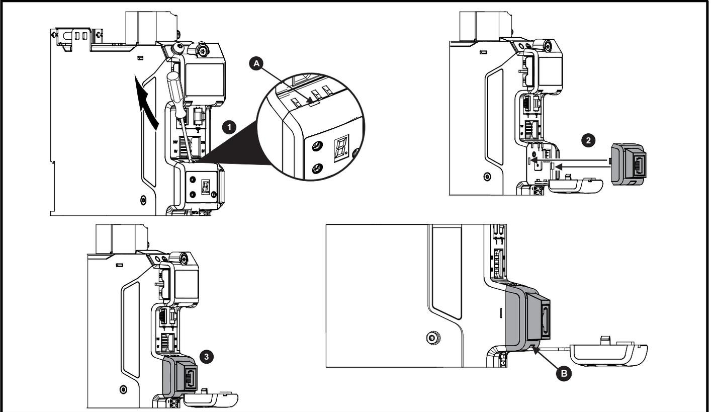
1. Unclip and pull the display away from the front cover. The tether keeps the display associated to the drive and should not be removed. A small terminal screwdriver maybe required to unclip the display. A slot in the drive plastic is provided for this purpose (A).
