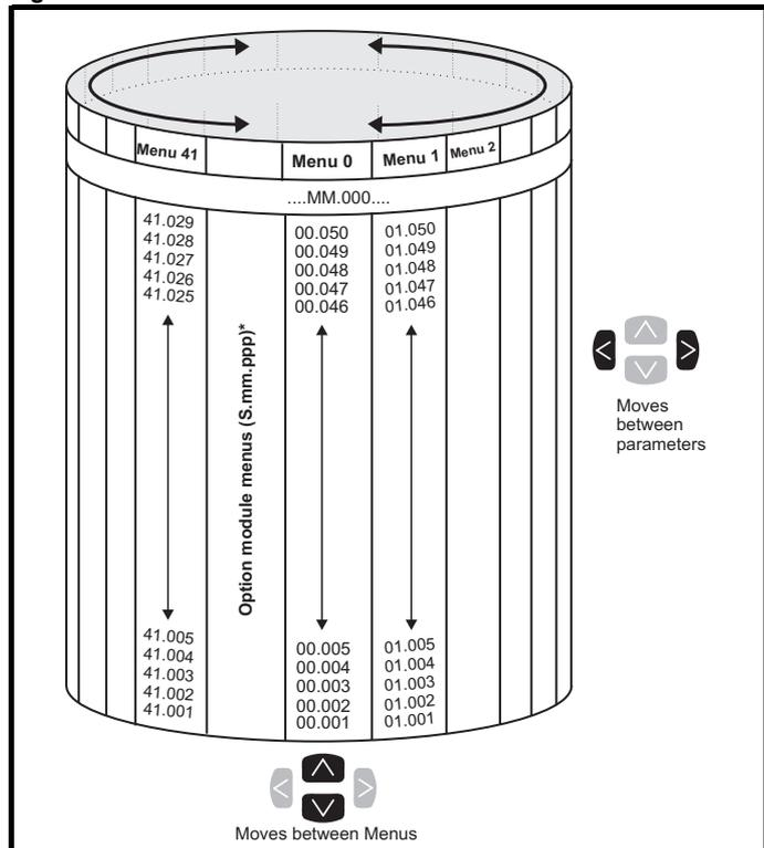
\* The option module menus (S.mm.ppp) are only displayed if option modules are installed. Where S signifies the option module slot number and the mm.ppp signifies the menu and the parameter number of the option module's internal menus and parameter.
