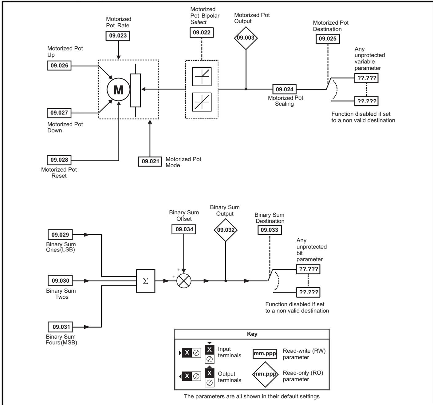
Figure 12-23 Menu 9 logic diagram: Timers
