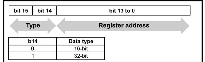
If 32-bit data type is selected then this effectively adds 16384 (0x4000) to the start register address.
