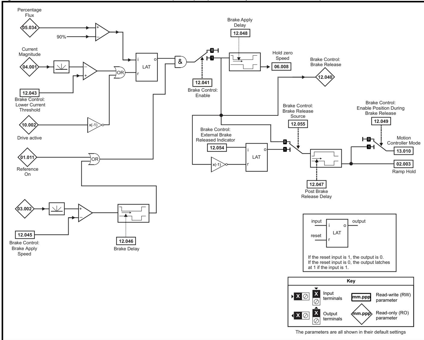
**Figure 12-30 RFC-A with position feedback brake sequence**
