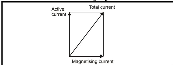
The active current is the torque producing current and the reactive current is the magnetizing or flux-producing current.
