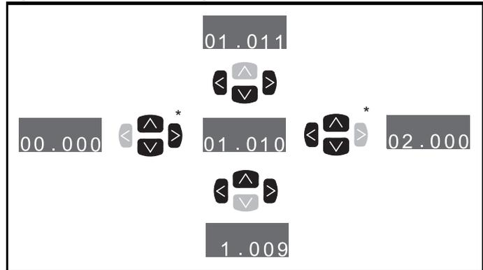
\* Can only be used to move between menus if all menus have been enabled (Pr **00.049**). Refer to section 5.9 *Parameter access level and security* on page 38.
