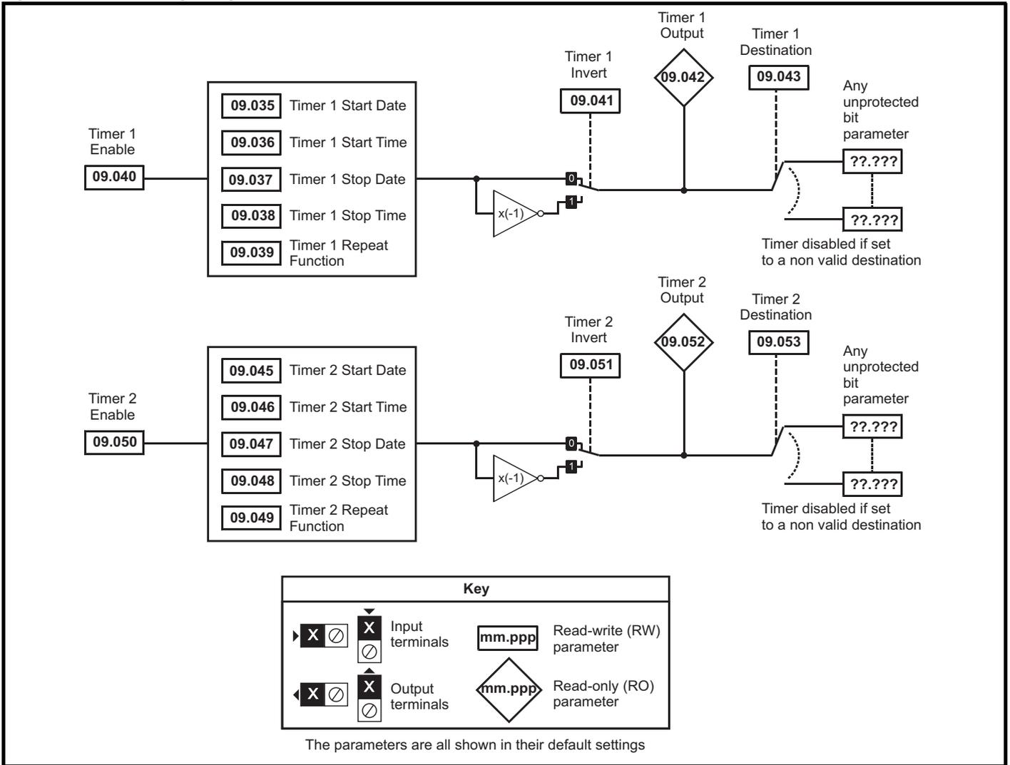
**Figure 12-24 Menu 9 logic diagram: Scope function**
