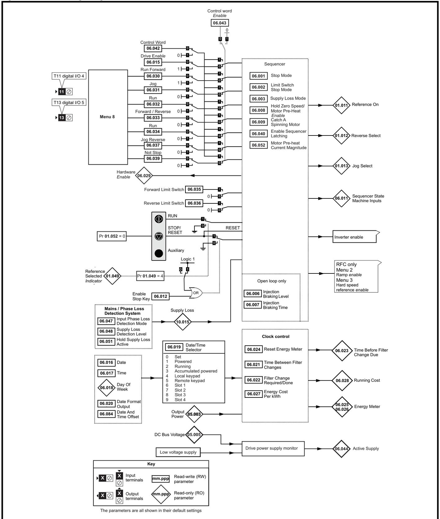
Figure 12-16 Menu 6 logic diagram: Under voltage and power supply control
