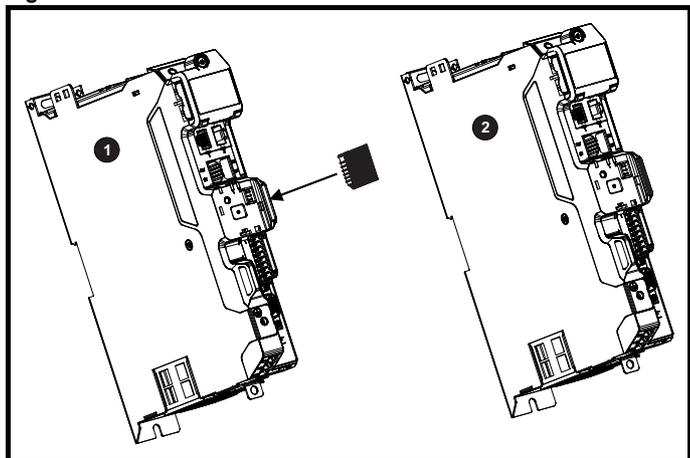
1. Installing the SD Card
