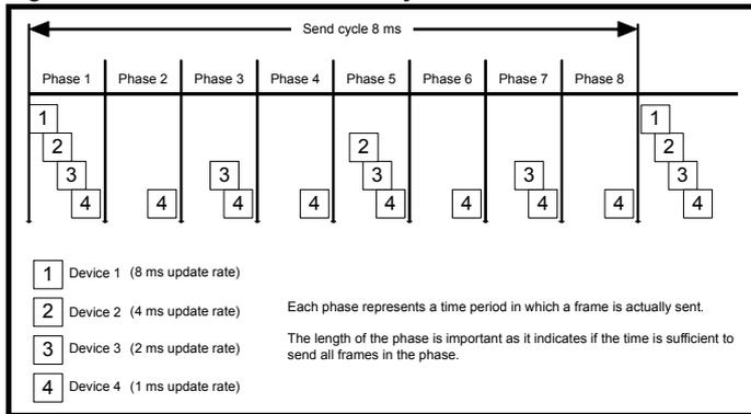
The Profinet transmission cycle is effectively the slowest update rate (8 ms in this example), and the phase duration is effectively the quickest update rate (1 ms in this example).
