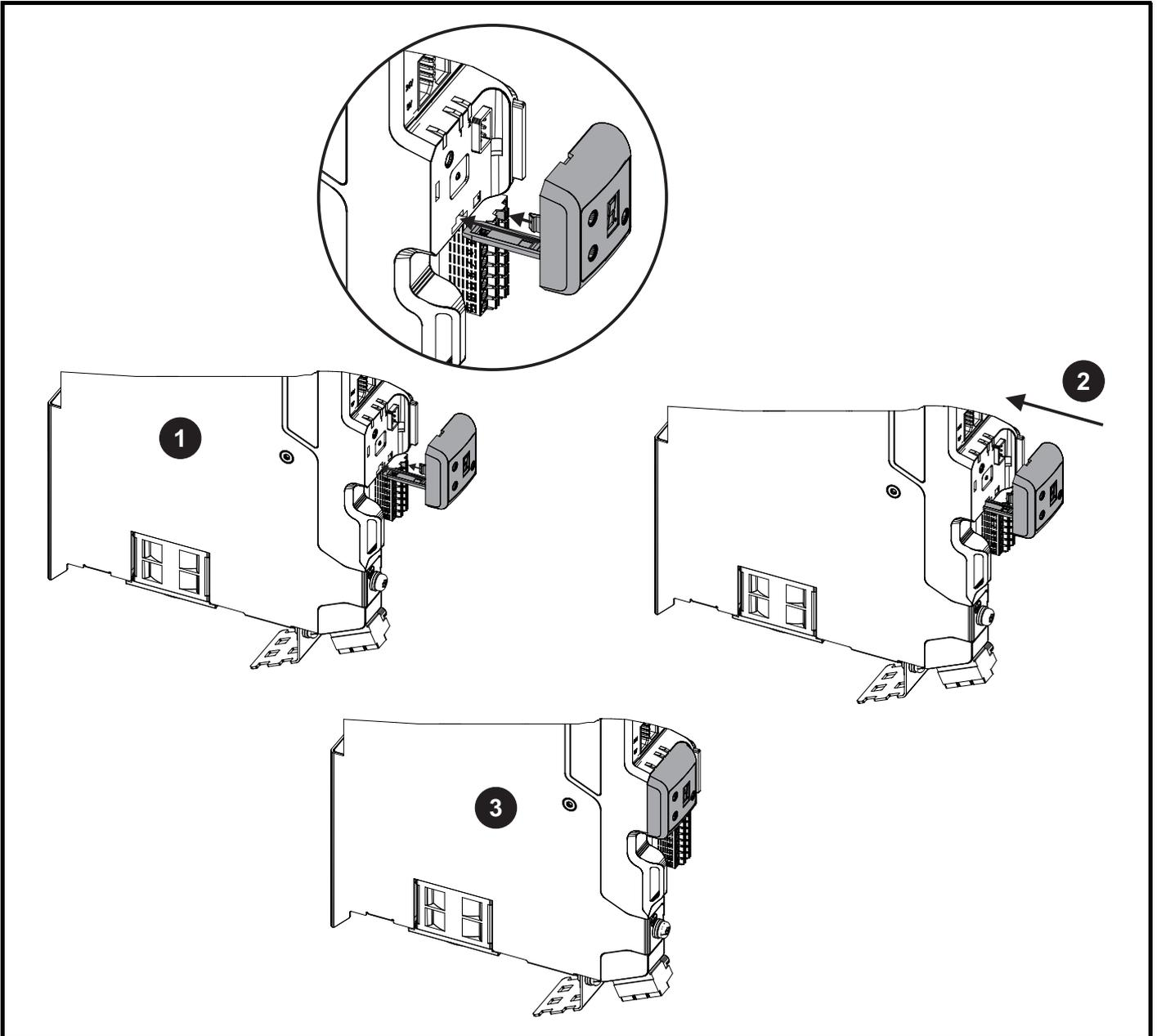
1. Align display tether with slot.
