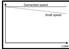
In order to prevent the speed droop shown above slip compensation should be enabled. To enable slip compensation Pr **05.027** must be set to a 1 (this is the default setting), and the motor rated speed must be entered in Pr **00.045** (Pr **05.008**).
