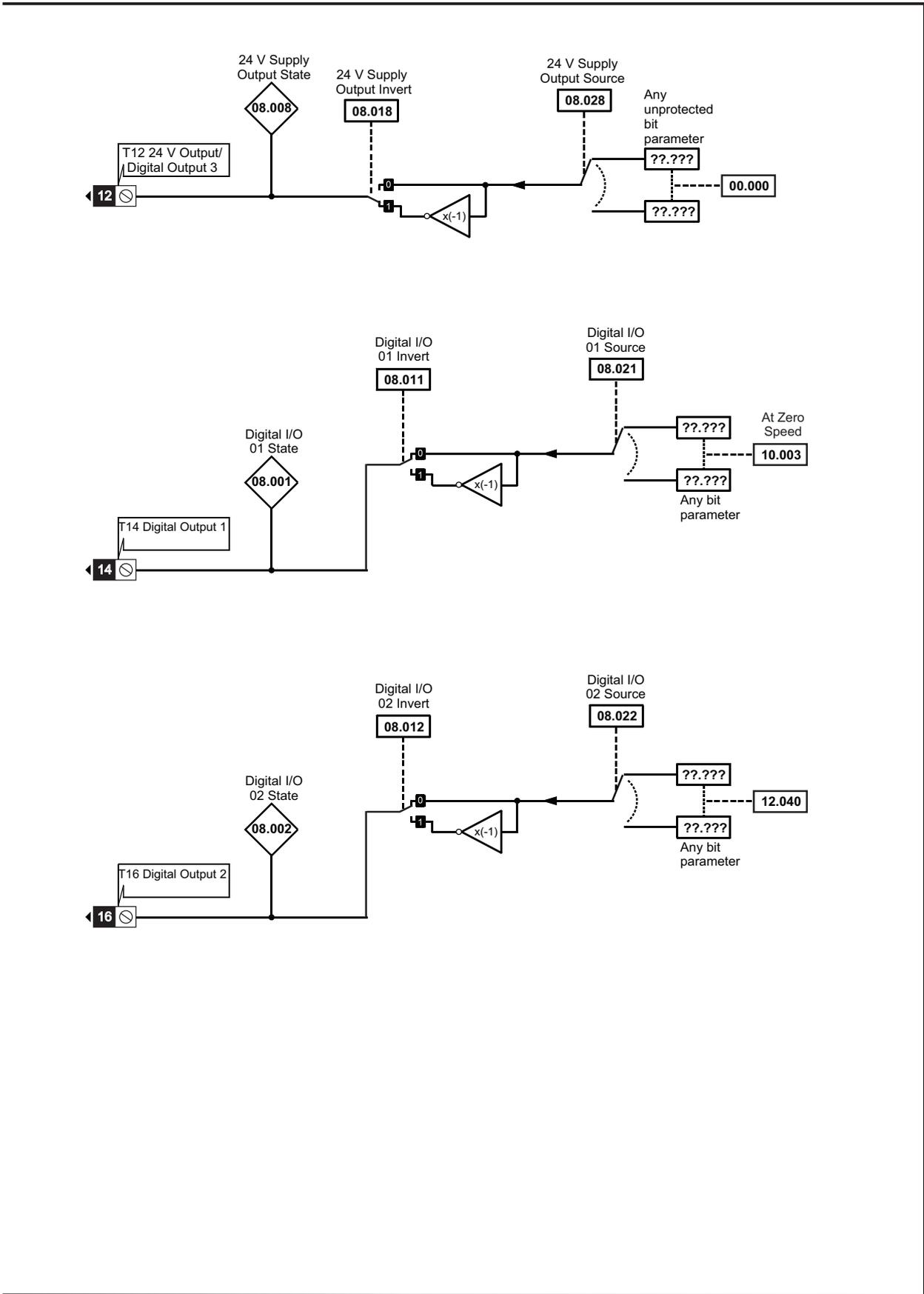
**Figure 12-20 Menu 8 Remote Keypad RTC buttons logic diagram**
