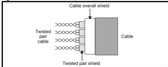
Using this type of cable also allows for the connection of the outer shield to ground and the inner shields to 0V alone at both drive and encoder end, when required.
