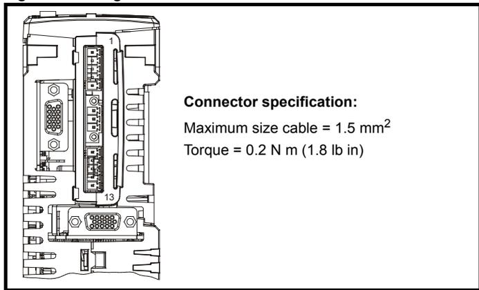
The terminals are numbered from terminal 1 at the top, to terminal 13 at the bottom as per the orientation shown in Figure 4-18. The terminal functions are given in Table 4-25:
