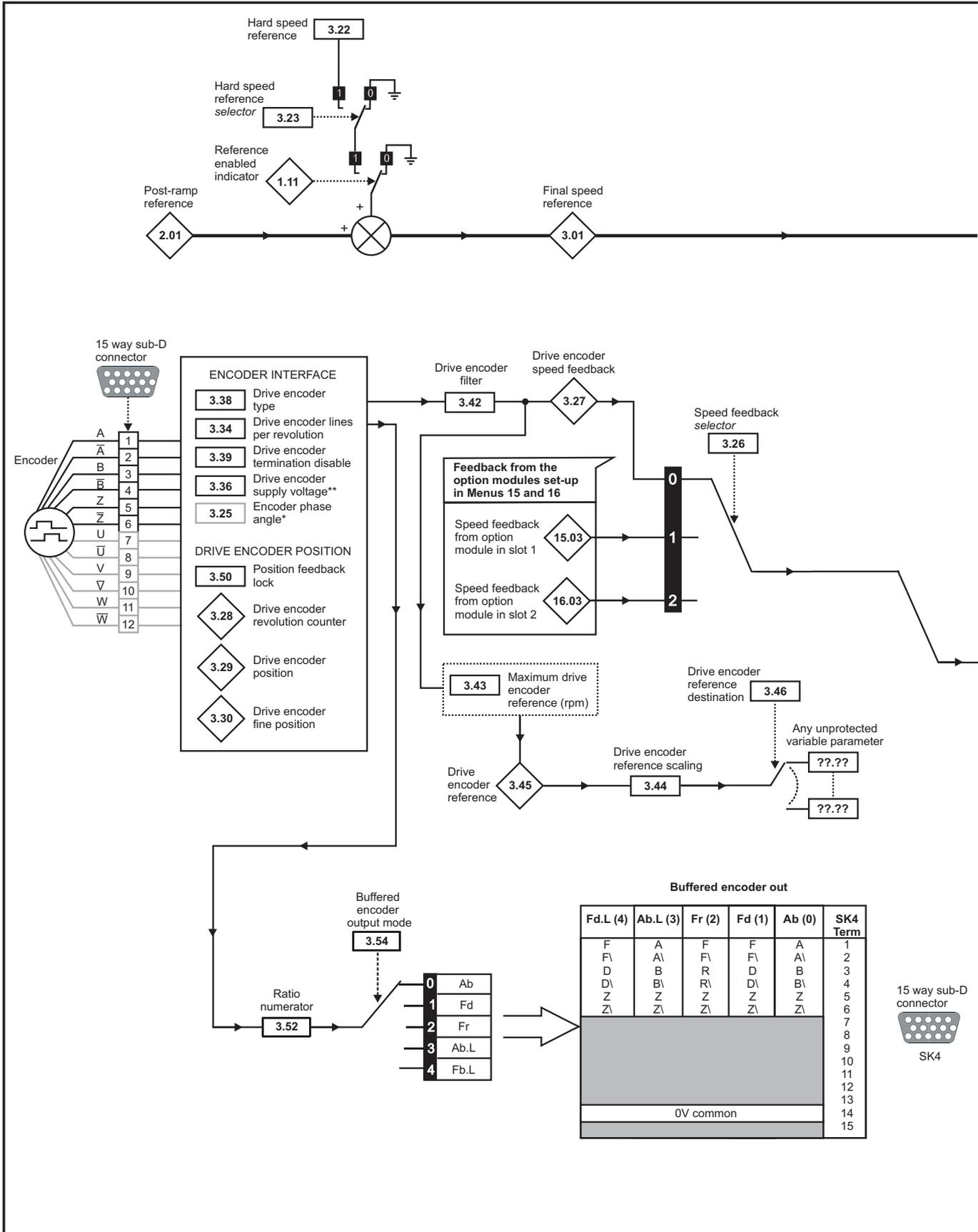
**NOTE** \*\*If Ab encoder voltage is greater than 5 V, then the termination resistors must be disabled Pr 3.39 to 0.
