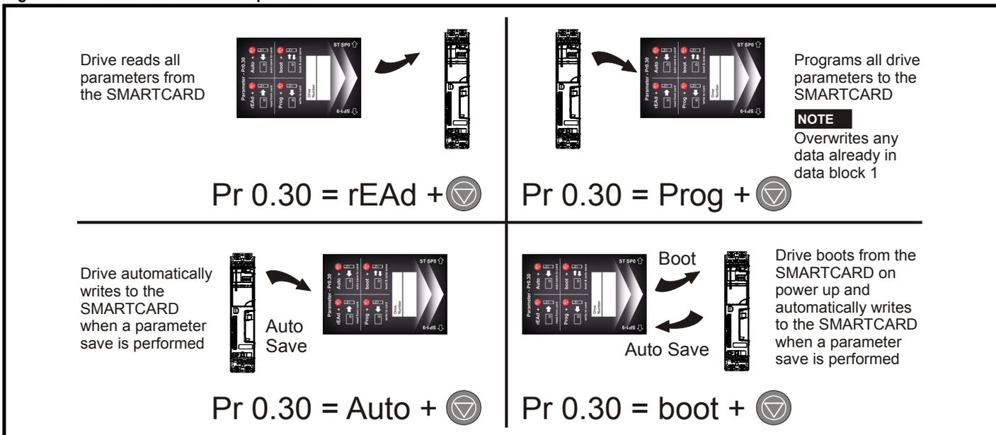
The SMARTCARD has 999 individual data block locations. Each individual location from 1 to 499 can be used to store data until the capacity of the SMARTCARD is used. The drive can support SMARTCARDS with a capacity of between 4kB and 512kB.
