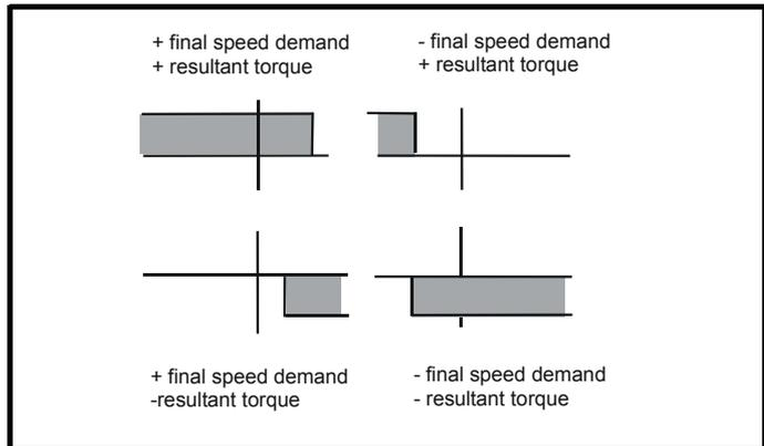
This mode of operation can be used where torque control is required, but the maximum speed must be limited by the drive.
