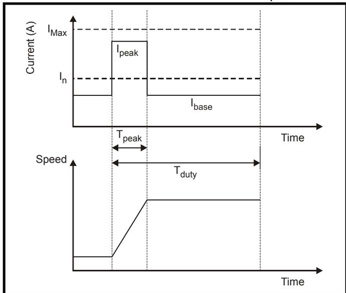
This is a profile with acceleration/deceleration periods where the peak output current from the drive ( $I_{peak}$ ) is given as a proportion of the nominal current ( $I_n$ ) for a defined period of time. ( $T_{peak}$ ).
