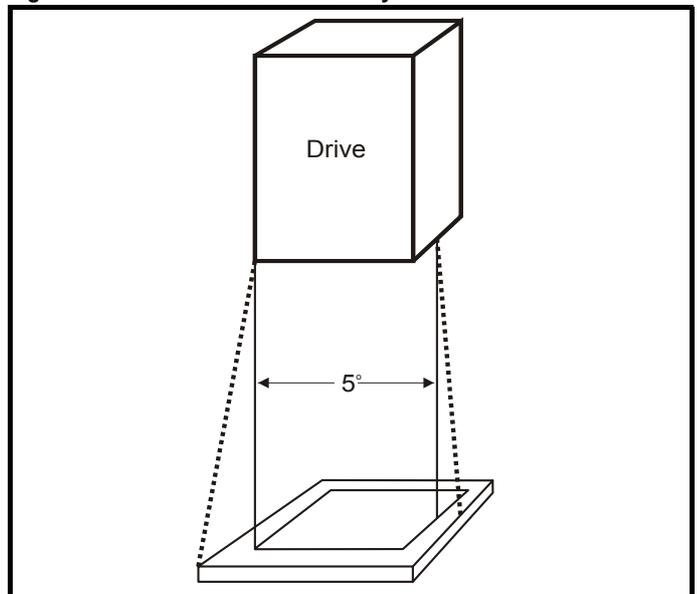
The bottom, including the part of the side considered to be part of the bottom, must be designed to prevent escape of burning material - either by having no openings or by having a baffle construction. This means that openings for cables etc. must be sealed with materials meeting the 5VB requirement, or else have a baffle above. See Figure 3-2 for acceptable baffle construction. This does not apply for mounting in an enclosed electrical operating area (restricted access) with concrete floor.
