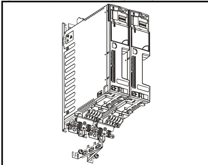
If installing multiple drives, one grounding bracket can be used for two drives.
