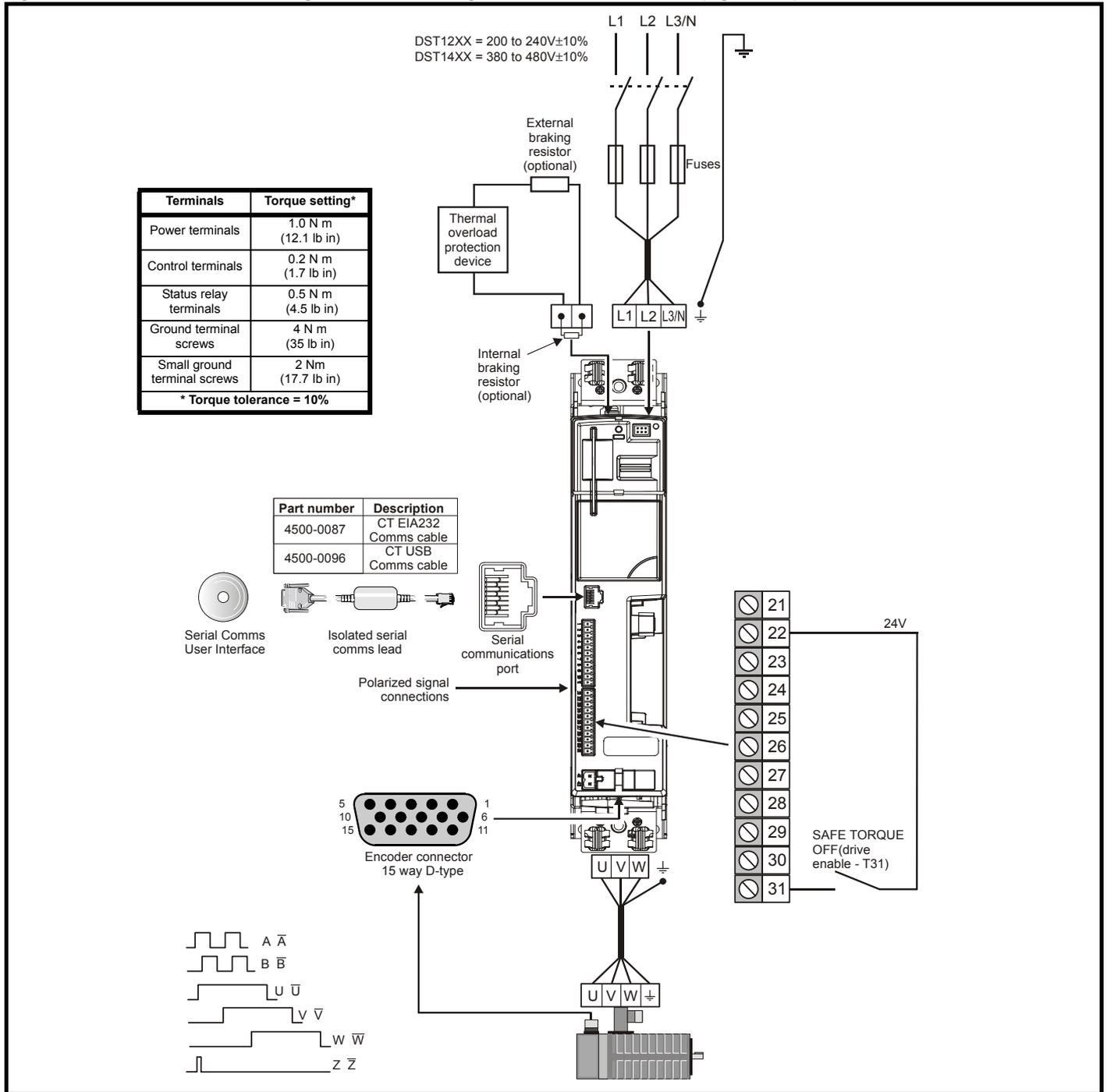
**Figure 7-2 Minimum connections to get the motor running via keypad**
