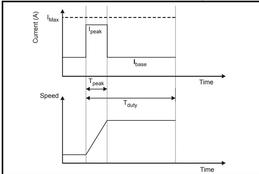
This is a profile with acceleration/deceleration periods where the peak output current from the drive ( $I_{peak}$ ) is given as a proportion of the base current ( $I_{base}$ ) for a defined period of time. ( $T_{peak}$ ).
