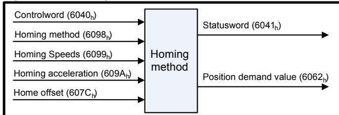
By choosing a homing method the following behavior is determined: The homing signal (positive limit switch, negative limit switch, home switch), the direction of actuation and where appropriate the position of the index pulse.
