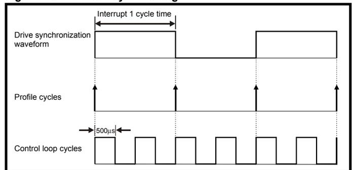
It is expected that most systems will have the interpolation cycle time equal to the drive synchronization interval. An interpolation cycle is referred to as a profile cycle. The inter-operation between a profile cycle when interpolation position mode is being used and the drive synchronization interval is described as follows:
