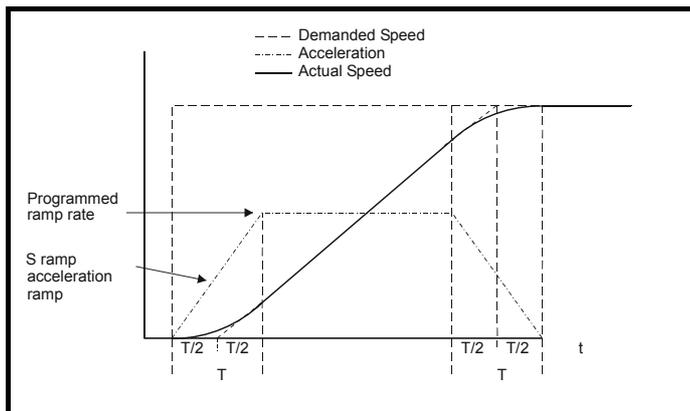
Since the ramp rate is defined in s/100 Hz or s/1000 rpm and the S ramp parameter is defined in s<sup>2</sup>/100 Hz or s<sup>2</sup>/1000 rpm, the time T for the 'curved' part of the S can be determined from:
