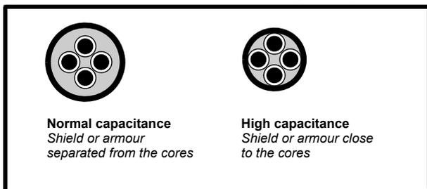
The cable used for Table 4-9 is shielded and contains four cores. Typical capacitance for this type of cable is 130 pF/m (i.e. from one core to all others and the shield connected together).
