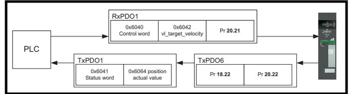
RxPDO1, TxPDO1 and TxPDO6 will need to be enabled in the master. Once enabled you will need to add mappings to the PDOs.
