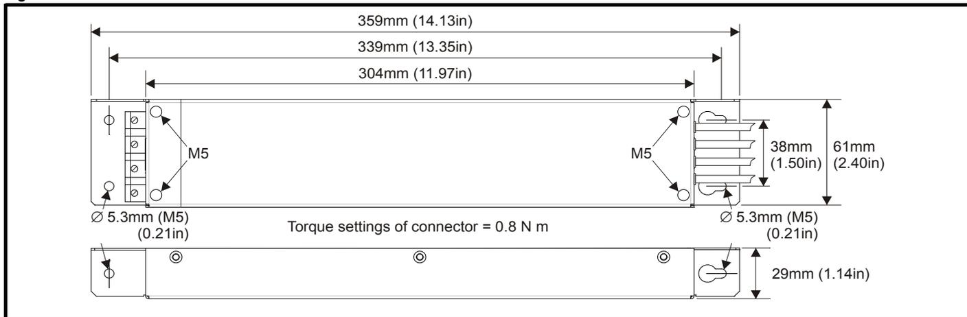
Figure 3-11 shows a 3 phase filter. For a single phase filter, there are only 3 input terminals (L1, N, ground) and 3 output cables (L1, N, ground).
