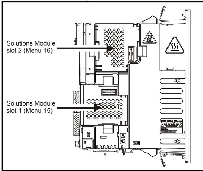
Pr 15.01 and Pr 16.01 indicate the type of module that is installed in the corresponding slot.
