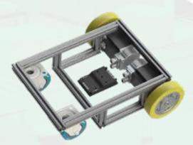
AGV's need two motors to move and steer. At Motion Control we can make this work with a single controller. Compared to the traditional One Motor/One Controller approach, the Dual Channel is simpler, cheaper, safer and easier to integrate and maintain. Two controllers can even team up to drive 4 motors with Mecanum wheels to move Omnidirectional Robots.
